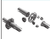
Metall-Vorder-/Hinter- differential (2 Stück)
